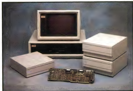
5 across SCSI technology that can be daisy-chained for up to 4 gigabytes of storage. 90, 180, 300, 600 MB capacities; 16-18 ms.*
